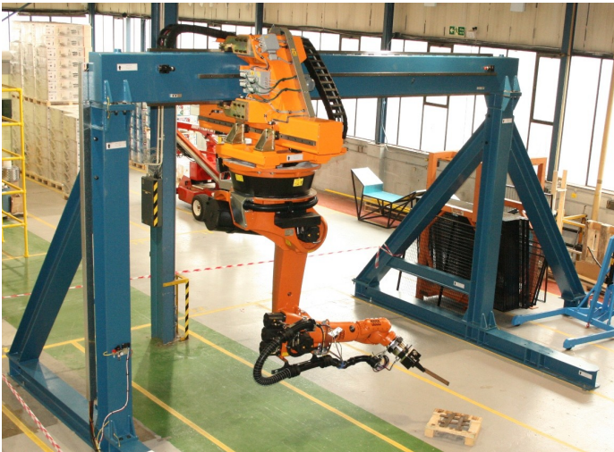
Waste sorting & size reduction test facility
